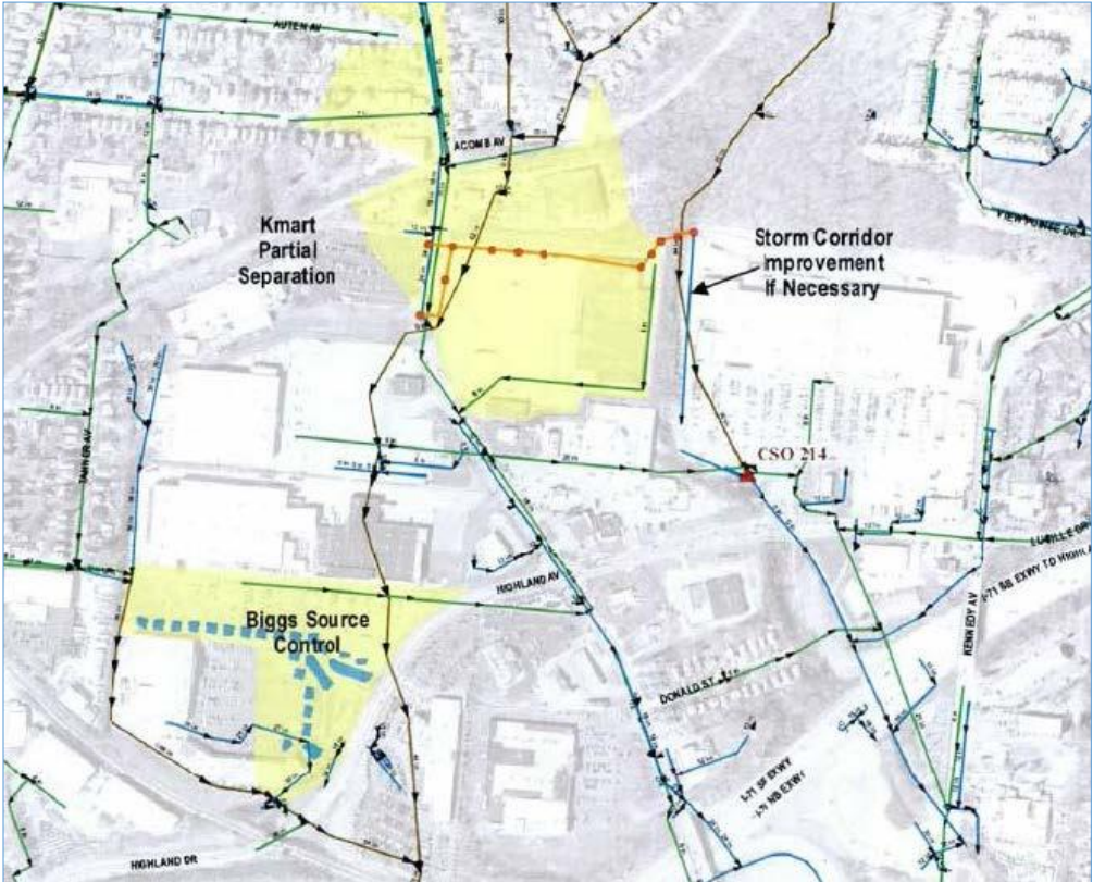
Figure 2. Proposed CSO 552 Stormwater Removal Project
